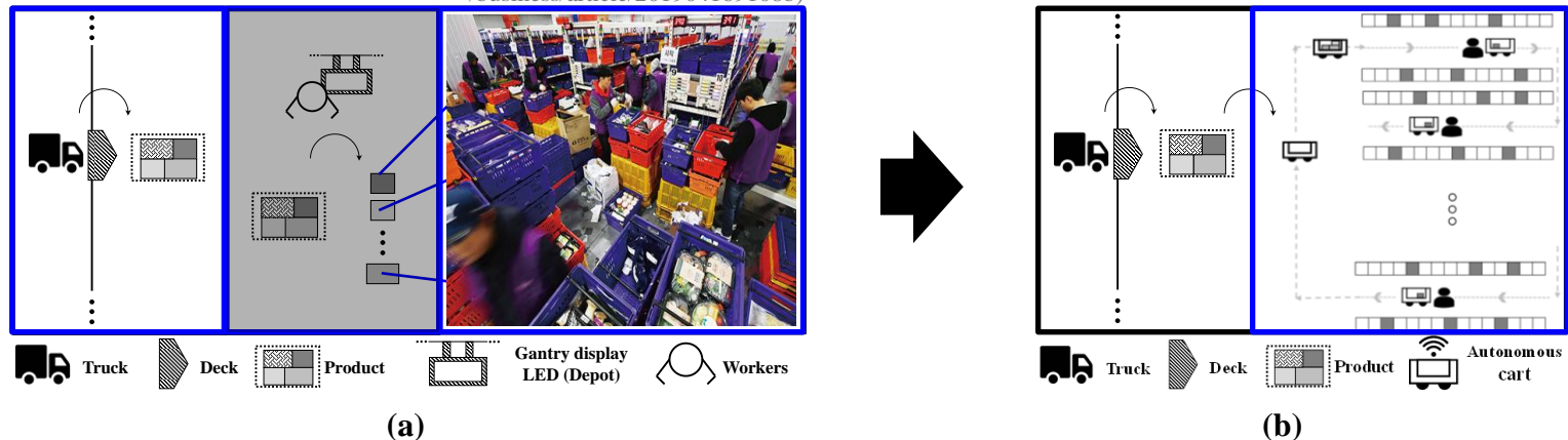
Figure 2. Technologies in the digital assorting system (modified from Lee et al. (2019)): (a) PTL and (b) Worker-following carts
